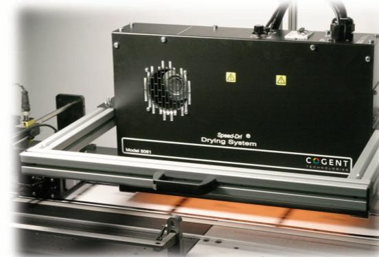
The Speed-Dri Model 5061 provides instantaneous infrared and convection technologies to dry ink printed on target areas up to 4" (102 mm) wide. Depending on the application, web speeds of up to 500 feet/min. can be achieved.
